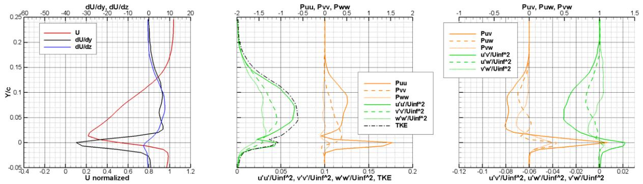
Figure 3. Variation of (a)  $U$ ,  $\partial U/\partial y$  and  $\partial U/\partial z$ ; (b) TKE, normal Reynolds stresses and production terms; (c) shear Reynolds stresses and production terms.
