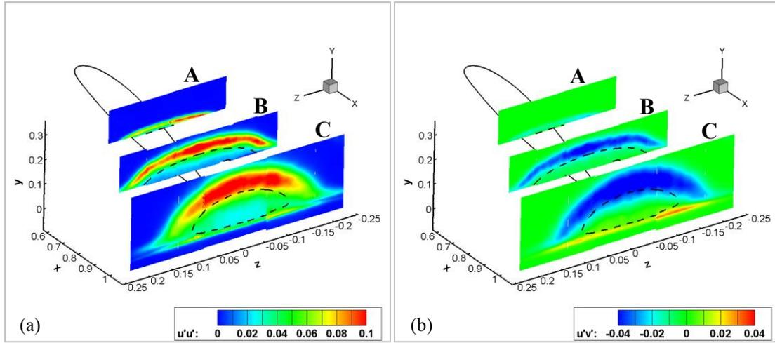
Figure 2. Contours of (a)  $\overline{u'u'}/U_\infty^2$  Reynolds Stress; (b)  $\overline{u'v'}/U_\infty^2$  Reynolds Stress on planes A, B and C.
