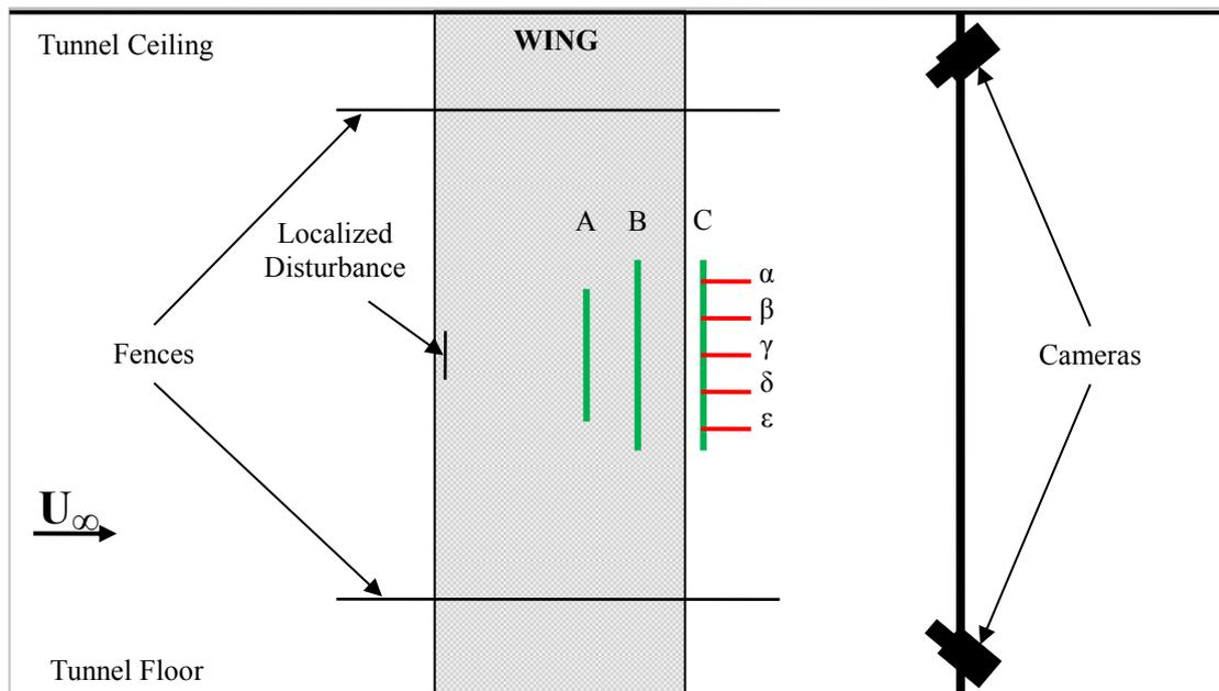
**Figure 1.** Schematic planform view of the test set up showing the wing, the fences, the stabilizing disturbance and the Stereo PIV cameras along with the measurement planes. Planes normal to the flow (A, B and C) are indicated by vertical green lines, while planes normal to the wing span ( $\alpha$ ,  $\beta$ ,  $\gamma$ ,  $\delta$  and  $\epsilon$ ) are shown with red horizontal lines.
