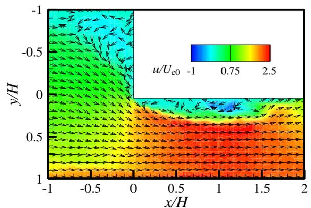
Figure 2. An instantaneous velocity field by PIV
