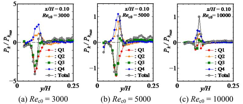
Figure 6. Quadrant analysis of the production term by PIV data
