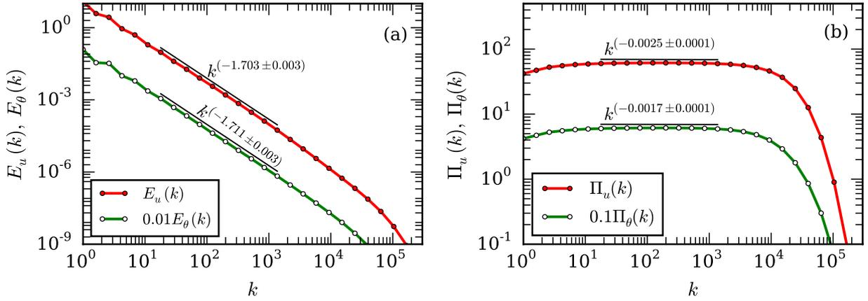
**Figure 2.** For convective turbulence simulation with  $Pr = 1$  and  $Ra = 10^{12}$ : (a) plots of KE and entropy spectra; (b) plots of KE flux  $\Pi_u(k)$  and entropy flux  $\Pi_\theta(k)$ .
