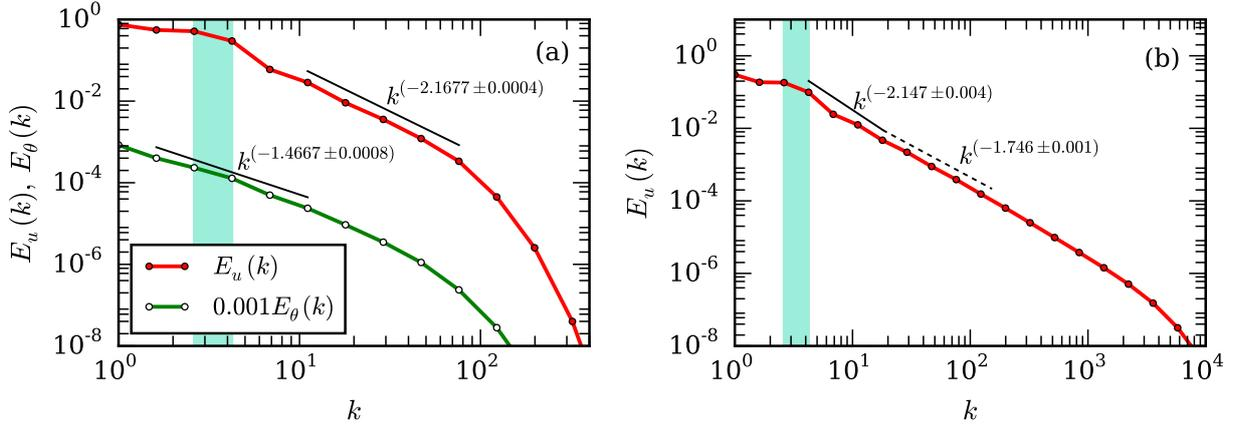
**Figure 1.** For stably stratified simulation: (a) plots of KE and entropy spectra for  $Pr = 1$ ,  $Ra = 10^5$ , and  $Ri = 0.10$  and (b) plot of KE spectrum for  $Pr = 1$ ,  $Ra = 10^{10}$ , and  $Ri = 0.25$ . In Fig. (b), the wavenumber range  $4 < k < 18$  exhibit Bolgiano scaling, and  $18 < k < 100$  exhibit Kolmogorov scaling (thus dual scaling). The green shaded region shows the forcing range.
