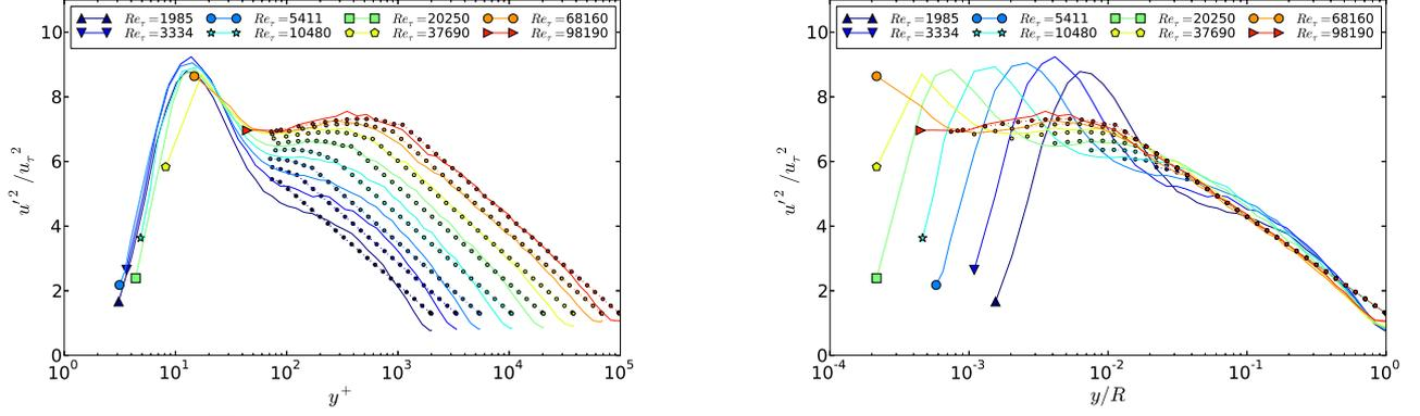
**Figure 1.** Plots of  $\overline{u'^2}(y)/u_\tau^2$  versus  $y^+$  (left) and  $y/\delta$  (right) obtained from the NSTAP Superpipe data of [3, 4] for different values of  $Re_\tau$ . The circles are calculated for all Reynolds numbers from equations (3) and (2) with  $y_* = \delta A^{1/p} Re_\tau^{-q/p}$  and  $A = 0.2$ ,  $C_0 = 1.28$ ,  $m = 0.37$ ,  $q = 0.79$ ,  $p = 2.38$  and  $\alpha = 1.21$ .
