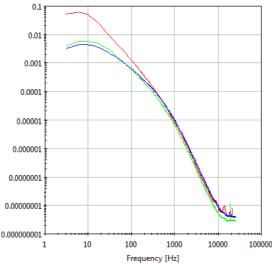
Figure 2. PSD for each velocity component (u-, v-, w-), at x=300mm and 42mm from the jet axis. References
