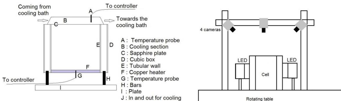
Figure 1. Convection cell (left) – cameras positioning (right).
