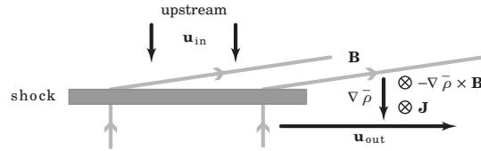
**Figure 2.** Slow mode MHD shock configuration and contribution of the oblique mean magnetic field and density gradient,  $\mathbf{B} \times \nabla \bar{\rho}$ , to the turbulent electromotive force (EMF).  $\mathbf{u}_{in}$  and  $\mathbf{u}_{out}$  are the in- and out-flow velocities, respectively.
