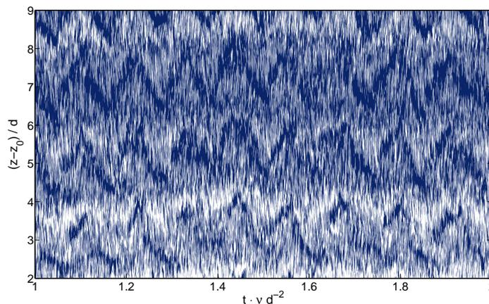
**Figure 1.** Space time diagram of a Taylor-Couette flow with  $Re_S = 5000$  and  $\mu = -0.2$  [4].
