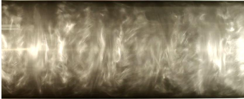
**Figure 2.** Photograph of a Taylor-Couette flow with  $Re_S = 5000$  and  $\mu = -0.2$ .
