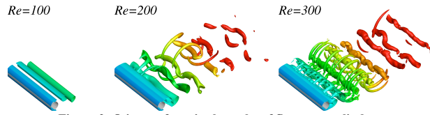
Figure 2: Q iso-surfaces in the wake of flow over cylinders.
