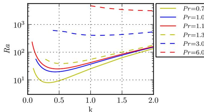
**Figure 1.** Stability curve of the laminar state for  $Re = 0$  and different values of the Prandtl number.
