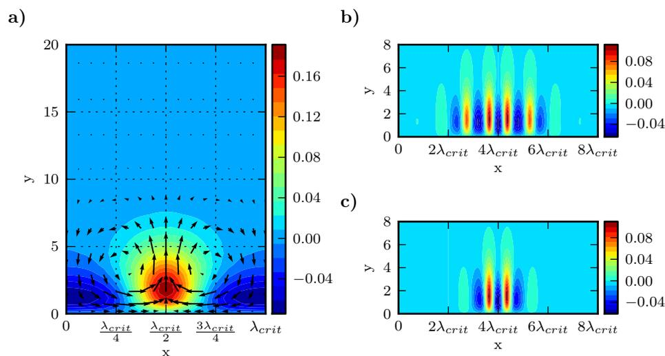
**Figure 2.** Flow- and temperature fields for the lower branch of the bifurcating roll-solution are shown in a). The flowfield is visualized by the arrows and the temperature is color coded. The Rayleigh number is 13, the Prandtl number is 1.0 and the spanwise wavelength is  $k_{crit} = 0.4305$ . In b) and c) the temperature field for two different spatially localized solutions is shown. In both cases the Rayleigh number is 17.8.
