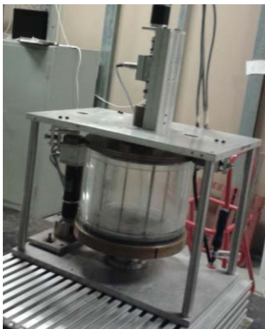
Figure 1. Picture of the Taylor-Couette setup.
