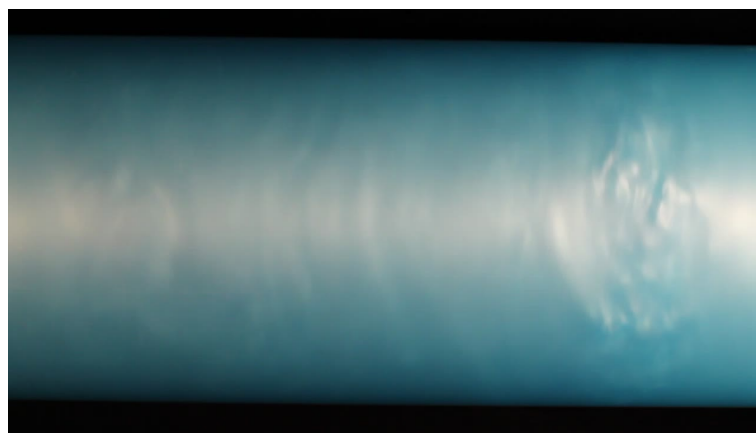
Figure 1. Turbulent spot for strong counter rotating wide gap Taylor-Couette flow ( \eta = 0.3 , Re_S = 12,000 , \mu = -0.4 )
