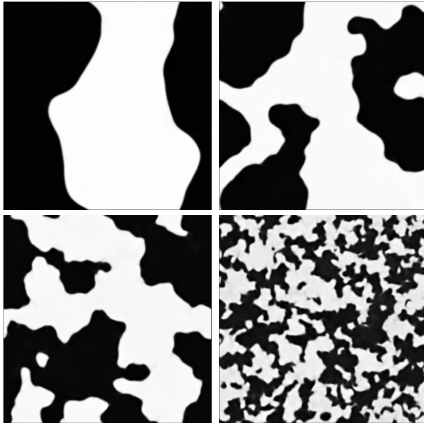
Figure 1. Pseudocolor plots of the order parameter field in the inverse-cascade regime in a two-dimensional turbulent binary-fluid mixture with increasing Weber number We = 1.2 \cdot 10^{-2} (top left), We = 5.9 \cdot 10^{-2} (top right), We = 1.2 \cdot 10^{-1} (bottom left), and We = 5.9 \cdot 10^{-1} (bottom right).
