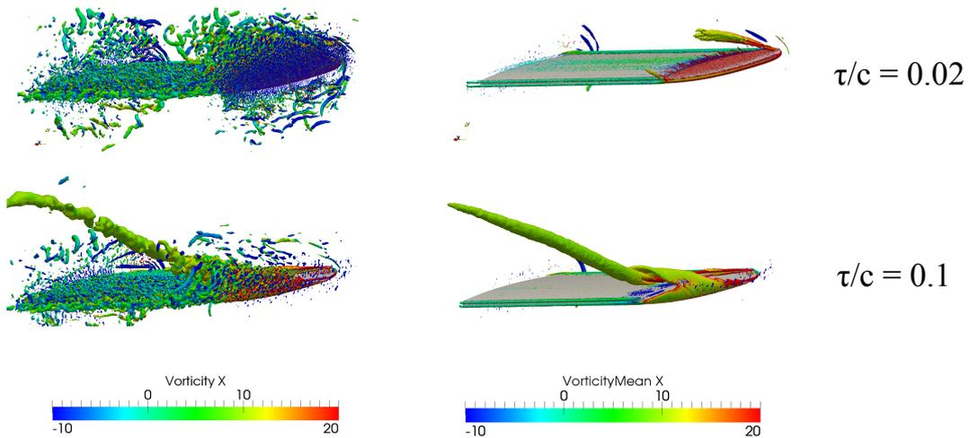
**Figure 2.** Q-criterion computed using the instantaneous velocity (left) and the mean velocity (right). LES computations.
