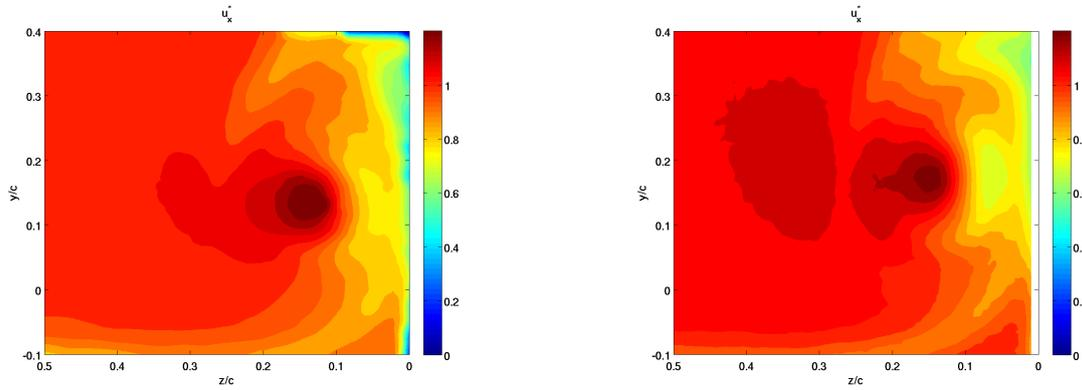
**Figure 1.** Axial velocity component  $u$  in a cross-plane downstream the blade for  $\tau/c = 0.1$ . Experiment (left), LES computation (right).
