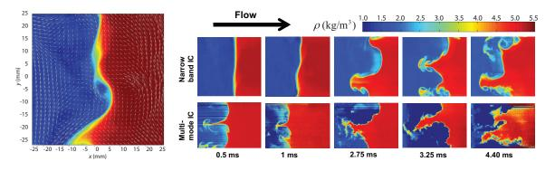
**Figure 1.** Left: Typical example of a simultaneous measurement of velocity (vector field) and density (contour map) at the initial conditions before shock. Right: Examples of the evolution of two initial conditions shocked at M=1.3. The top series is for a narrow-band initial condition and the bottom series is for a multi-mode initial condition. Each column represents a different stage of evolution after shock interaction. Only contour maps of density are shown for simplicity.
