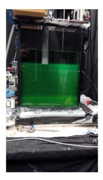
Figure 1. Picture of the experimental apparatus. Vortex rings are generated at the base of the grey tube within the tank. The dye intensity corresponds to the fluid salt concentration.
