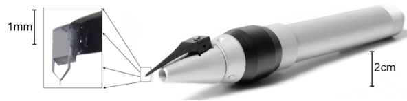
Figure 1. Illustration of the 2d-Laser Cantilever Anemometer with detailed view of the tip section and cantilever.
