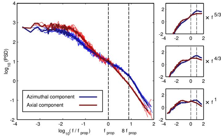
**Figure 2.** Left: Spectral density for all the considered experimental runs. Right, the same data compensated by different powers of the frequency (indicated in the pictures).
