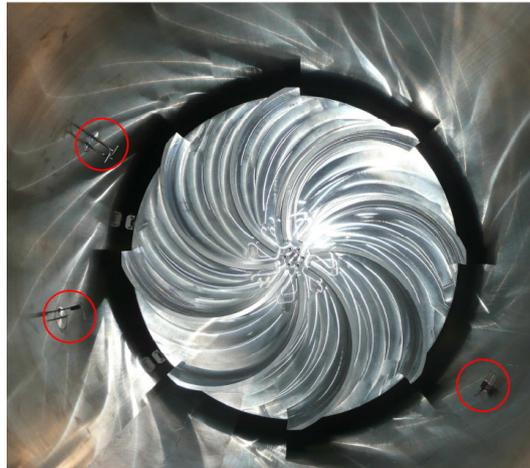
**Figure 1.** Top view of the experimental cell: the bottom propeller (the top propeller has been removed) and the different velocity probes (marked with red circles) around the middle plane of the cylindrical wall are visible. In this contribution we present the results corresponding to the Pitot tubes on the top left. See the text for a detailed explanation.
