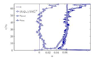
Figure 1. Decomposed turbulent entrainment coefficient in a steady jet at Re = 6815.
