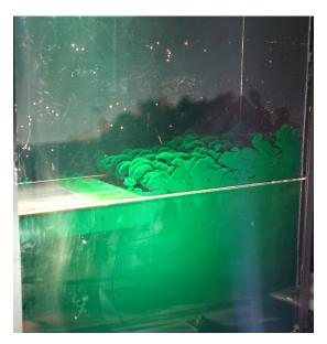
Figure 1: Perspex tank used in experiments with the stainless steel barrier left partially in. The lower layer is dyed with fluorescein and food dye to make it appear solid. The 3D growth of the RTI instability is clearly seen as are the initial stages of the circulation in the upper layer with undyed fluid seen to be moving off the edge of the barrier into the opening.
