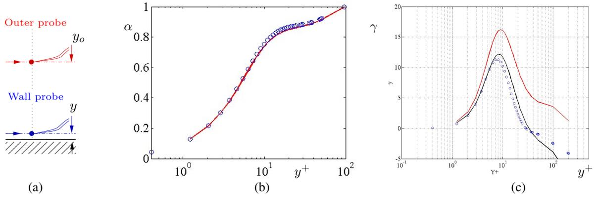
**Figure 1.** Probe setup (a); coefficients  $\alpha_u(y^+)$  (b) and  $\gamma(y^+)$  (c) as given by the theory (line) and numerical simulation (points).
