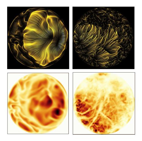
Figure 1. Field lines of the skin friction field (top row) and the vertical temperature derivative (bottom) taken at the wall of the cylindrical convection cell at z=0. The left column shows convection in air at a Pr=0.7, the right column in a liquid metal Pr=0.021. Both data records are obtained at  $Ra=10^8$ . The largest magnitude of the temperature derivatives is found in the dark colored regions. The brightest regions are the lowest magnitude and hence are regions of plume detachment.
