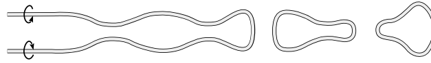
Figure 1. Sketch of the Crow instability in which anti-parallel vortex filaments develop into vortex rings through reconnection in an ordinary fluid with finite viscosity. Reproduced from Ref. [2].
