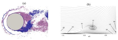
**Figure 1.** Overview of the flow field. Top view of isosurfaces of the Q-field at two instances in time (with different colours) (a) and streamlines of the time average velocity field in front of the cylinder (b).
