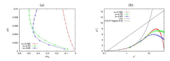
Figure 2. Velocity profile in the symmetry plane in front of the cylinder at three different positions of x in outer scaling (a) and in inner scaling (b).
